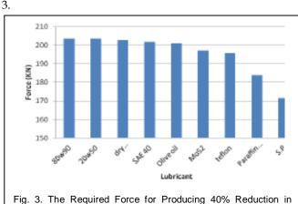
Fig. 3. The Required Force for Producing 40% Reduction in Height in Stainless steel Specimens.
