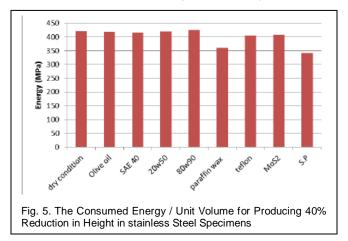
On the whole, it can be concluded that the use of S.P as solid lubricant is the most effective lubricant among the other lubricants. This is explicitly indicated in figures 6 and 7. Die steel, D2. It can be seen from Fig. 6 (a) to (e) inclusive, which indicate the amount of barreling after compression for identical D2 specimens for using S.P, SAE 40, olive oil and the dry condition, and for MoS2 respectively. For the three lubricants, the amount of barreling is almost the same and slightly less
