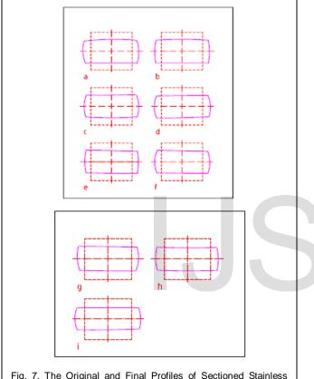
Fig. 7. The Original and Final Profiles of Sectioned Stainless Steel Specimens Using Different Lubricants where a, b, c, d, e, f, g, h, and i for Olive Oil, MoS2, 20W50, the Dry Condition, Teflon, 80W90, SAE 40, Superplastic Tin-lead Alloy, and Paraffin Wax Respectively
